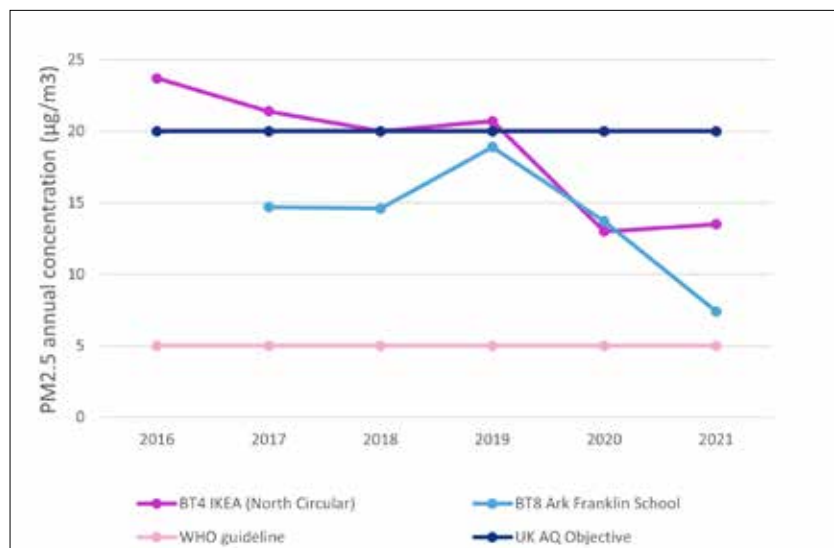
Figure 4: Annual Mean PM 2.5 Concentrations at BT4 (Ikea), and BT8 (Ark Franklin Primary School)
