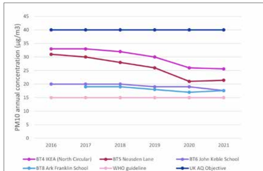
Figure 3: Annual Mean PM 10 Concentrations at BT4 (Ikea), BT5 (Neasden Lane), BT6 (John Keble Primary School), and BT8 (Ark Franklin Primary School)
